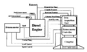
Fig. 1. A schematic diagram of the diesel engine test bench.
