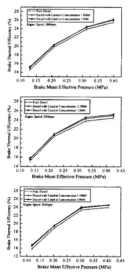
Fig. 5. The brake thermal efficiency as a function of the engine load (BMEP).
