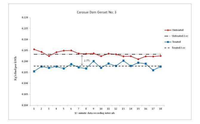
The efficiency gain of 8.6% recorded by the untreated test engine can only be a result of instrumentation malfunction. The net efficiency gain resulting from fuel treatment with the FTC-3 Catalyst is **2.7%**. Although this is at the lower end of efficiency normally achieved, it must be pointed out that this operation is a very well run station and engines were base loaded (locked in) during tests at their most efficient load of 0.8MW.
